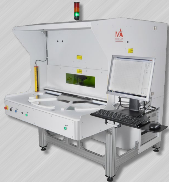
Laser marking workstation type XL with 50 W fibre laser Station designed with semi-automatic six positional rotating carousel, fitted with calibrated holes for replaceable insertion devices.
